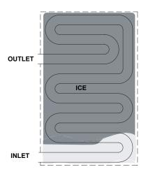
Figure 7-4. Extremely Thin Ice Formation at Evaporator Inlet
